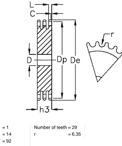
C = 1 D = 14 De = 92 Dp = 88.09 For chain size =  $3/8 \times 7/32$ For chain type = 06 B-3 h3 = 25.6 L = 5.2
